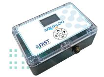
Latest generation RTU integrated in Cloud architecture is the innovative response for the monitoring and control of water distribution systems. This is a PRV and pump controller to regulate pressure in the districts, able to manage reduced leakage in the best way possible, with extended capacity to monitor connected sensors (pressure, temperature, level and quality).
