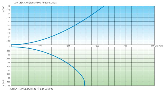
The air flow charts were created in Kg/s from laboratory tests and numerical analysis, then converted in Nm<sup>3</sup>/h using a safety factor.
