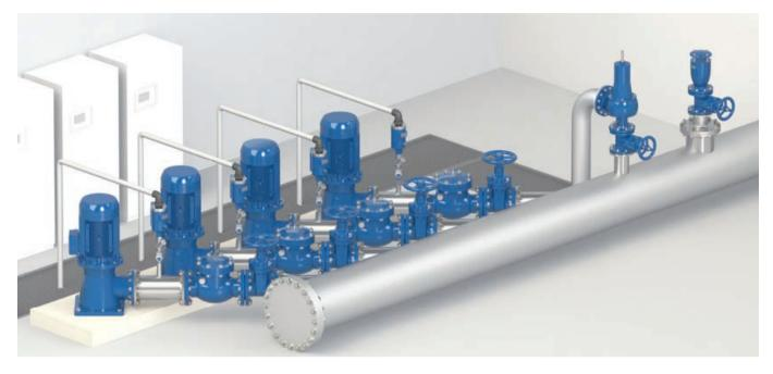
**Pressure reduction valve station.** In this second layout H-PVS 90F is installed downstream of a pressure reduction valve station to prevent in any case rise in pressure on the main line. The installation also includes the pressure reducing valve PF H-VAL 310/410, a by-pass for maintenance and anti-surge combination air valves WAVE or WAVE LITE 3S-AWH upstream and downstream.
