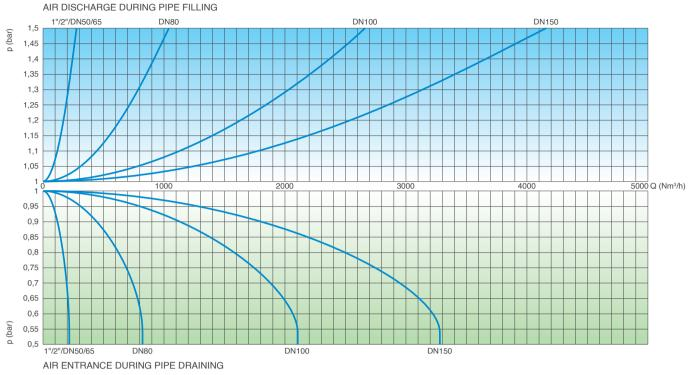
The air flow charts were created in Kg/s from laboratory tests and numerical analysis without the screen, then converted in Nm³/h using a safety factor.
